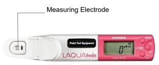
If the Measuring Electrode has not been used for a long period of time, or if the Electrode has been left extremely dry, then use this moistening procedure.
