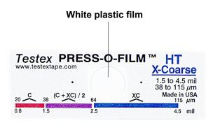
Remove the Testex Tape from the surface and place the replica between the anvils of the Testex Gauge, making sure that it is centred properly. Release the Testex Gauge anvil gently onto the replica and measure the profile. The gauge reading is the average maximum peak-to-valley height of the blast-cleaned surface.
